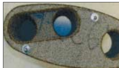
Fig. 2: Hollow spheres, integrated in the car exhaust pipe, can be used as silencers, optionally with catalyst effect. They are temperature resistant and easy to handle.
