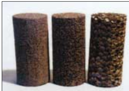
Fig. 1: New material structures made from differently sized metallic hollow spheres.
