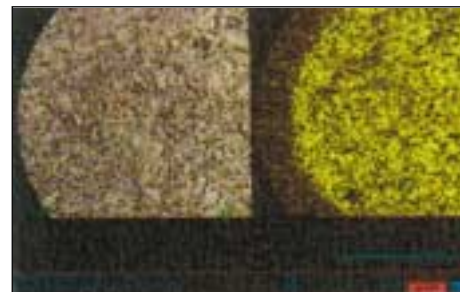
Fig. 3: Solid catalyst sphere Left: Unused catalyst Right: Used catalyst. The photo shows clearly, that only the outer darker shell has been reactive. The yellow core was not used. Consequently, a hollow sphere saves material and can save cost and increase reactivity due to the possibility to "engineer" the surface layer.
